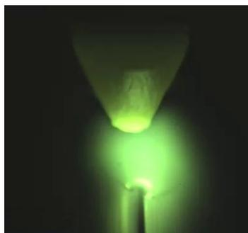
Figure 1: Magnified vision of welding pool and welding pool shapes, as well as the distance between the two metal strip edges. This information can be elaborated by visual processing to obtain precise and useful information parameters like:
